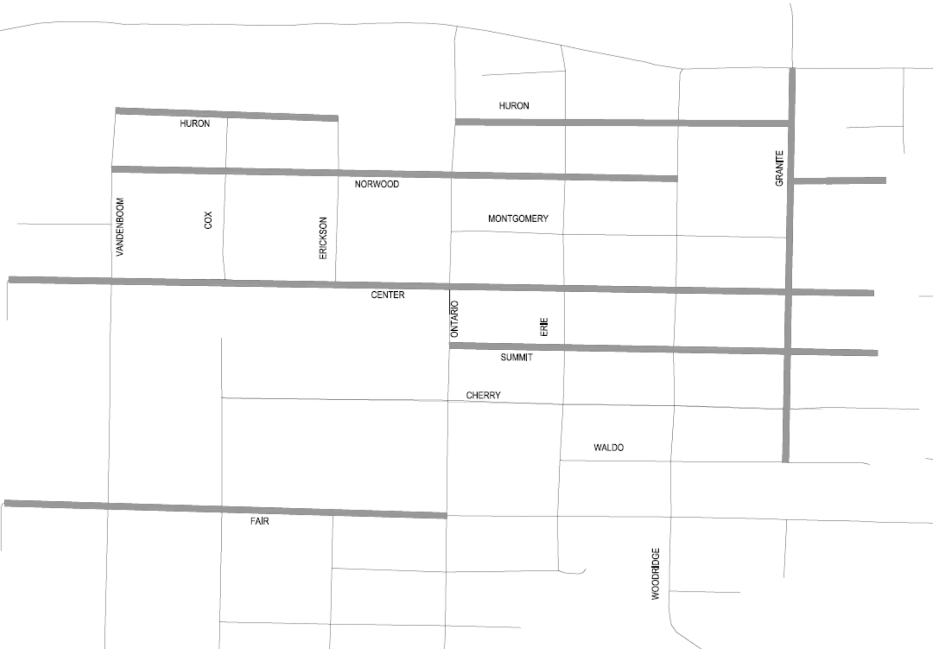
Figure 3: Trowbridge Park Area watermain replacement
